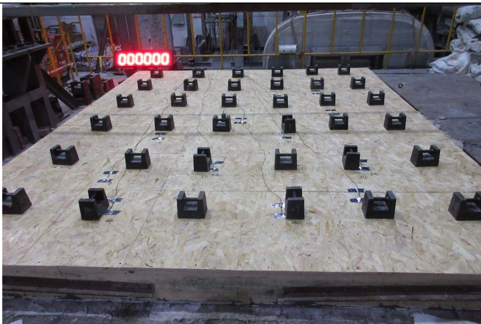
The unexposed face of the floor assembly before the test
